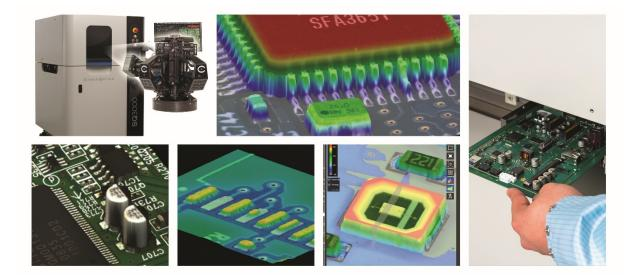
Powered by proprietary Multi-Reflection Suppression<sup>™</sup> (MRS<sup>™</sup>) sensor technology, the 3D SQ3000 all-inone system offers an unmatched combination of high speed, high resolution and high accuracy. The MRS sensor meticulously identifies and rejects reflections caused by shiny components making it an ideal technology solution for a wide range of applications, particularly high-end and challenging applications with stringent quality requirements.
